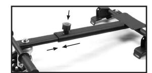
Step 2. Attach Control Handles (5) to the rear of the main chassis with Long Bolts & Nuts (A) using Allen Key (D) and Spanner (E).
