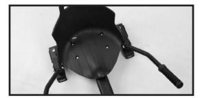
Step 4. Attach Hoverkart to a hoverboard under the seat using the Adjustable Straps (1).
